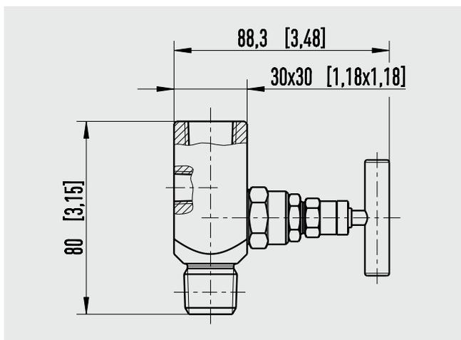
Plug screw for vent connection is included in delivery, though not pre-fitted.
