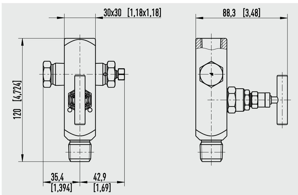
Plug screw and vent screw is included in delivery, though not pre-fitted.
